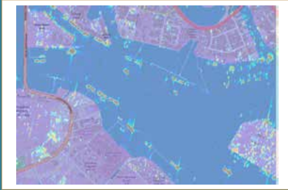
Ships detection results, overlaid on optical imagery using FBR (Frozen Background Reference) technique
